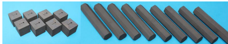
Fig. 11. MSD printed D185 green parts (left: cubes 20x20x20 mm 3 for slurry and workflow development; right: hexagonal beams with \varnothing_1 = 11 and L = 75 mm for mechanical testing in green and sintered state)
