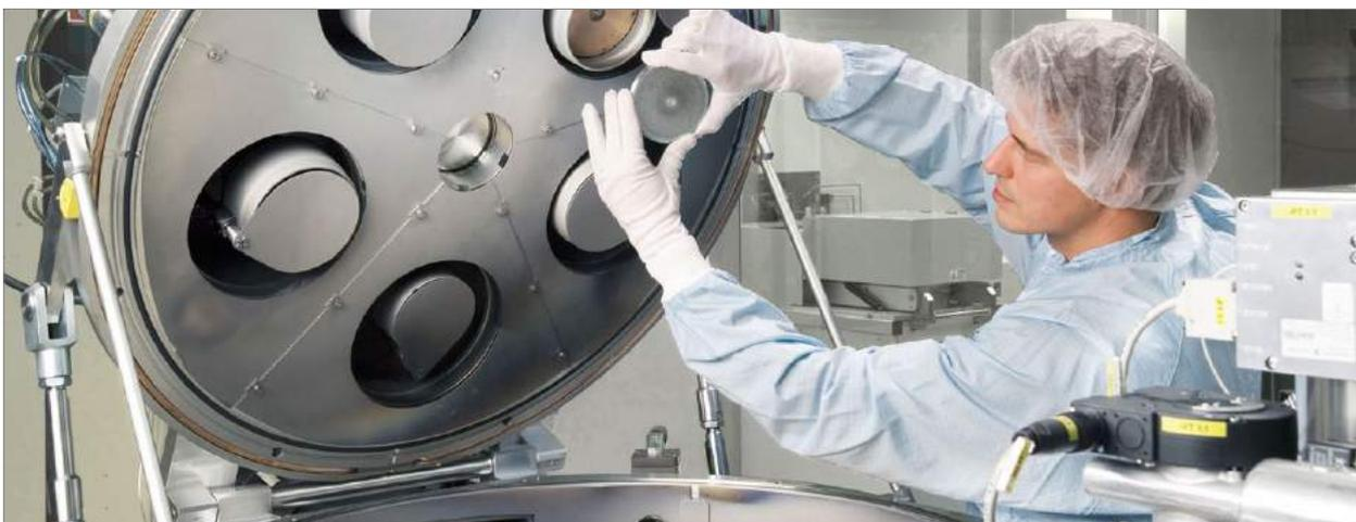
Fig. 1 Plansee's PVD application laboratory performs sputtering in near-real life conditions
