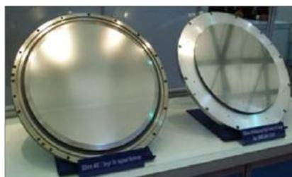
Ultra-high purity W targets for the semiconductor industry (hot pressing or hot isostatic pressing)
