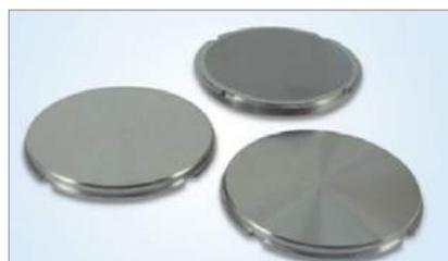
TiSi targets for hard coating applications (spark plasma sintering)
