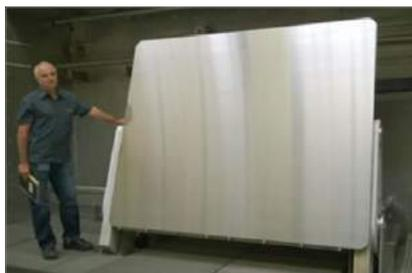
Large-size Mo planar target for the flat panel display industry (pressing & sintering, hot rolling)
