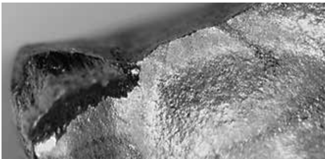
Excessive stress of the insert causes breakage.
