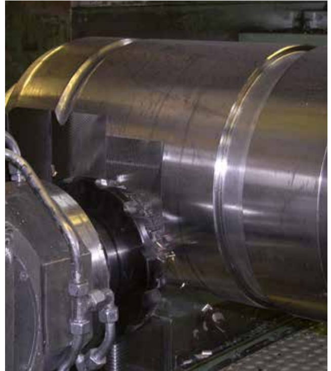
Stable and process-secure: machining large cast iron and steel rolls calls for robust, wear-resistant tools with high cutting depths.
