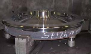
MACHINING THE HUB BORE
