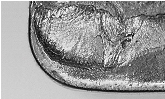
The outgoing hot chip is causing cratering of the cutting insert on the clamping surface.
