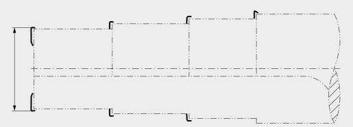
Boring Ø: 14 – 65 mm Boring indexable insert: SOEX / SOGX / WOEX / TOHX / TOHT ISO indexable inserts Step Ø: 17.5 – 65 mm, Step angle: 90° – 15° Step indexable insert: WOEX / SOEX / SOGX / TOHX / TOHT ISO indexable inserts
