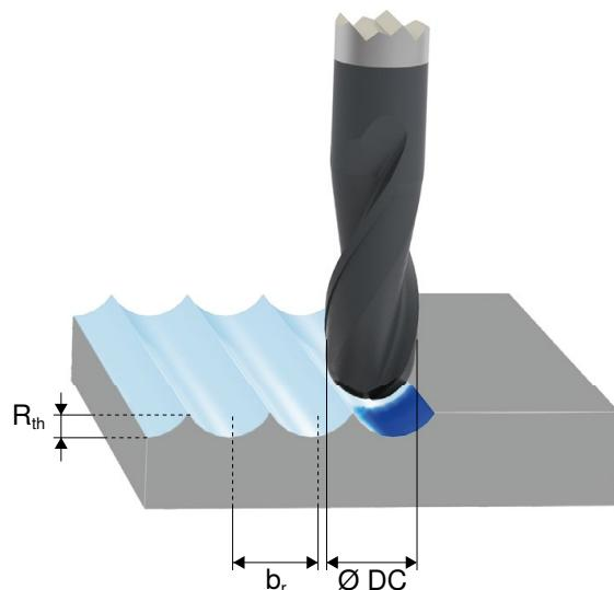
RPM correction factor (Kf n) for copy milling
