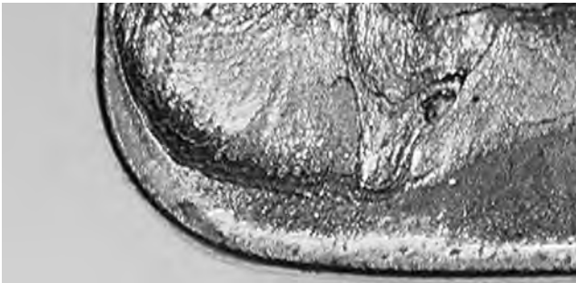
The hot chip which is being evacuated causes cratering at the rake face of the cutting edge.
