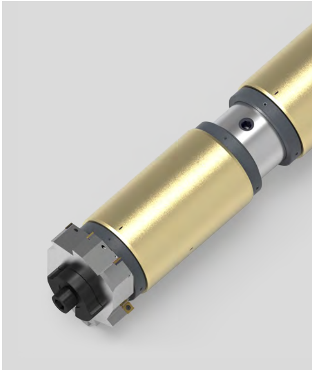
Reverse machining screw head on turbine housing \varnothing 189 mm
