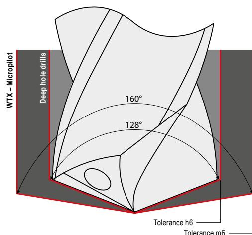
The following must apply to use the pilot and deep hole drill consecutively and without collisions:  $\Delta D = \text{ØD (pilot hole)} - \text{ØD (deep hole)} > 0$
