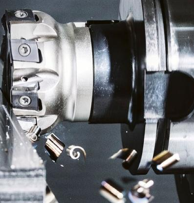
Side and face milling cutter system
