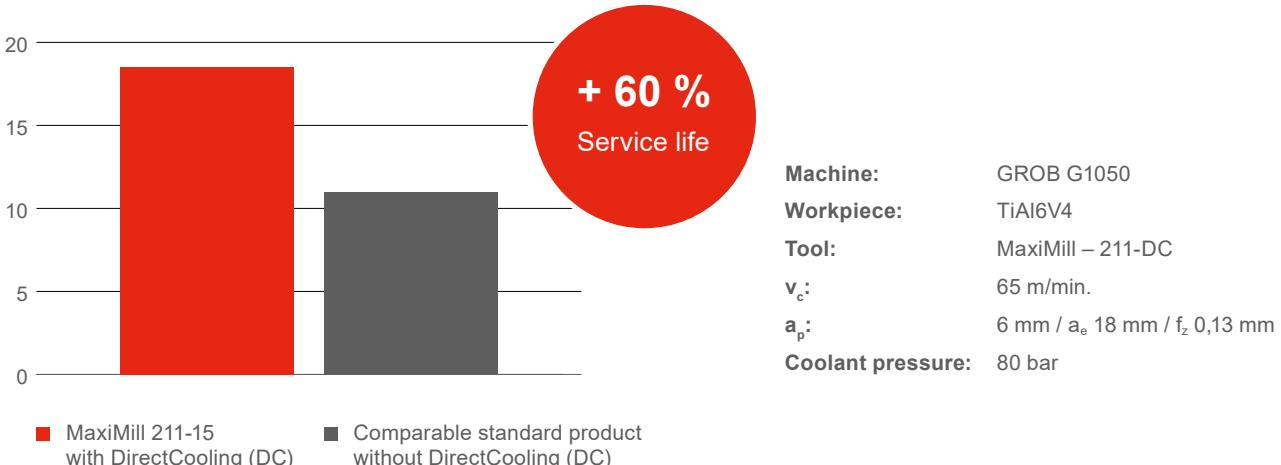
Having that extra time on the service life really takes the pressure off for our customers when machining titanium and super alloys. Plus, they benefit from a reliable process – with significantly lower tool usage.
