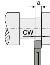
When grooving with an axial displacement the width „a“ should amount to at least 70 % of the grooving width „CW“.
