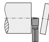
For parting pip-free, use R or L inserts. In order to minimize lateral deflection reduce feed by approx. 20–50 %.
