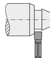
When grooving oblique surfaces the feed should be reduced by approx. 20–50 % until fully engaged.
