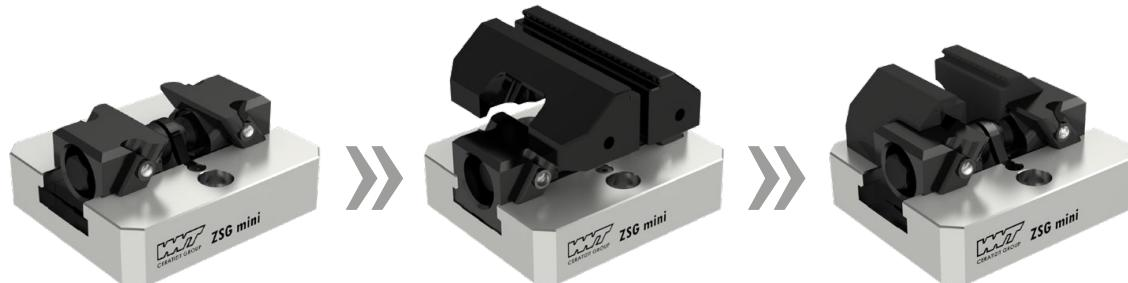
The jaws can be replaced in a matter of seconds without any tools at all by extracting them at an angle through the centre. The integrated pull-down action via two spring pressure pins means that the jaws sit securely in the base body, ensuring total machining precision and robust connections.
