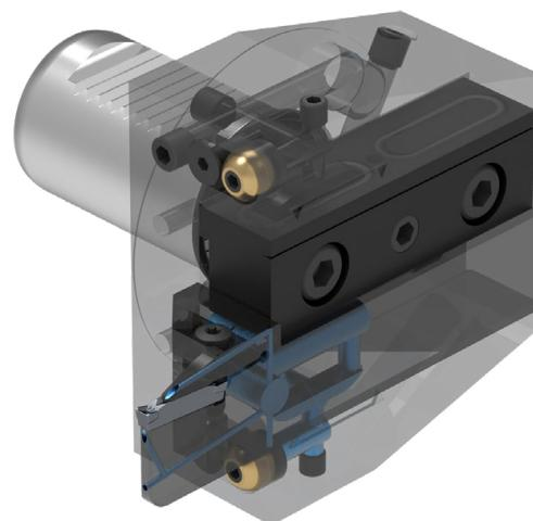
*The DirectCooling system from CERATIZIT optimises cooling lubrication: two coolant holes trained on the cutting edge ensure efficient cooling, lubrication and chip evacuation.*
