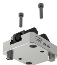
Clamping with two M6 screws from above through the base body. Alignment can be performed using Ø 12H7 precision holes.
