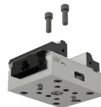
Dia. 12<sup>H7</sup> precision holes are present in all variants for positioning the ESG 5 with precision. All variants can be mounted with screws from above through the base body.
