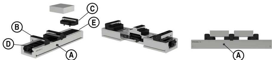
The lateral clamping screw A is not tightened, instead it is open approx. 1/2 turn. When the vice is fully open, the movable jaws B and C are to be placed in the appropriate slots of slides D and E and secured according to the workpiece size. Two workpieces of different sizes can also be clamped.
