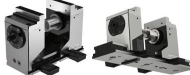
Alignment through 20<sup>H7</sup> precision slot nuts in the base body (H5G) and alignment sets 14 / 16 / 18 in the machine table's T-slot. Clamping with clamping claws.
