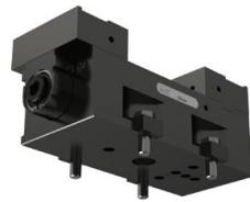
With clamping claws, the ESG mini 100 mm can be directly clamped on grid plates (50 mm x 50 mm) in a grid dimension of 100 mm x 100 mm or T-slot tables with 100 mm spacing.
