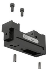
In the basic version, 2 dia. 8<sup>H7</sup> positioning holes are used for positioning. These can be used to align the ESG mini 40 mm on grid plates (**Article no. 80 897 944 and 80 897 946**) and machine tables with T-slot. The ESG mini 40 mm can be mounted from above with 2 M8 fixing screws.
