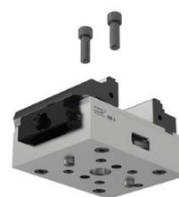
Dia. 12<sup>H7</sup> precision holes are present in all variants for positioning the ZSG 4 with precision. All variants can be mounted with screws from above through the base body.
