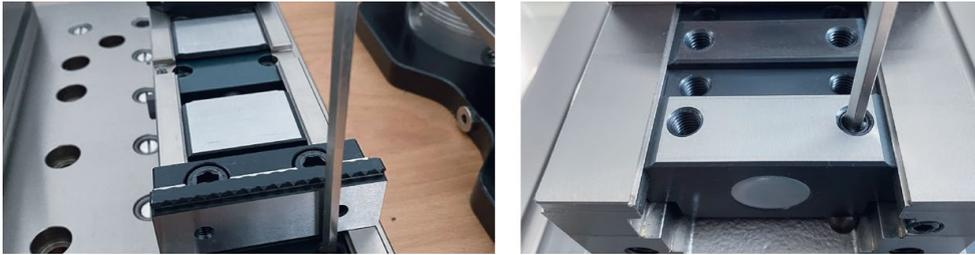
The rear slide is blocked via the hexagon socket grub screw and the DSG 4 can also be used as a single vice. **Important note:** Not suitable for using several vices as single vice next to one another. In this case, we advise modification with additional transverse slot in the base body and suitable fixed jaw.
