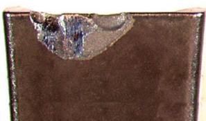
Excessive mechanical stress on the cutting edge causing carbide particles to break out.
