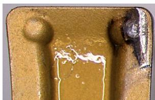
The outgoing hot chip causes cratering of the insert on the clamping surface.
