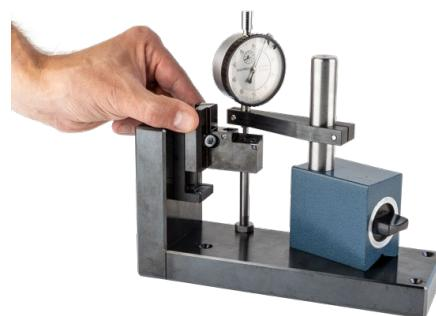
3. Carefully place the dial gauge on the tip of the tool's cutting edge.
