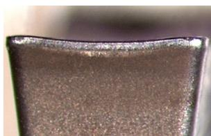
Abrasions on the flank, normal wear after a given operation time
