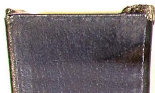
Weld deposits of material on the cutting edge occurs when the chip does not flow caused by low average temperature.
