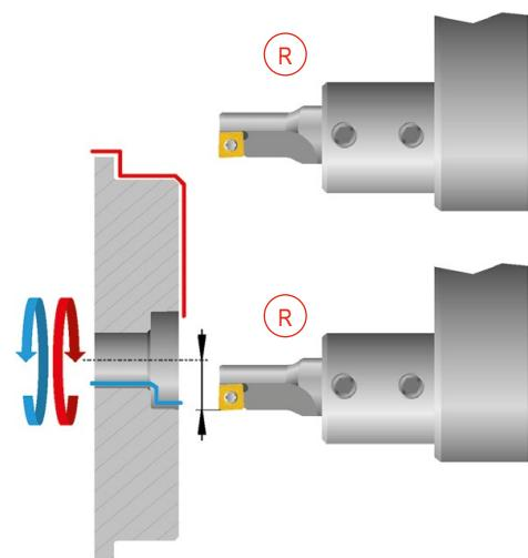
With axial displacement there is the danger of collision!
