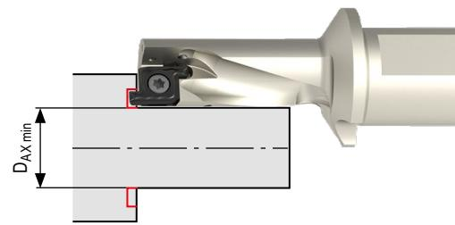
For maximum chip transport efficiency when drilling, coolant pressure must be 3–6 bar minimum (optimal 7–10 bar).
