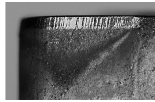
Wear on clearance face
