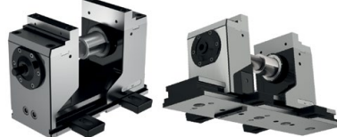
Alignment through 20 H7 precision slot nuts in the base body (H5G) and alignment sets 14 / 16 / 18 in the machine table's T-slot. Clamping with clamping claws.
