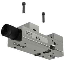
Clamping with two dowel screws dia. 12 H7 / M12 (NCG 100) Article no. 80 890 313 or dia. 16 H5 / M16 (NCG 125 / 160) Article no. 80 890 314
