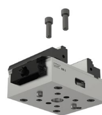
Dia. 12 JS precision holes are present in all variants for positioning the ZSG 4 with precision. All variants can be mounted with screws from above through the base body.
