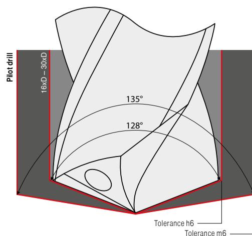
The following must apply to use the pilot and deep hole twist drill consecutively and without collisions:
