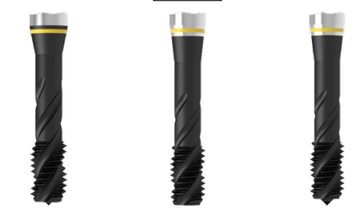
HSS-E FHA 42° ≤ 900 N/mm² ≤ 3xD HSS-E FHA 45° ≤ 900 N/mm² ≤ 3xD HSS-E FHA 45° ≤ 900 N/mm² ≤ 3xD
