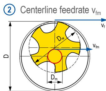
$$v_{fm} = \frac{v_f \times (D - D_w)}{D} \text{ mm/min.}$$
