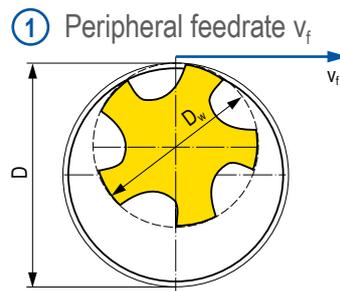
$$v_f = n \times f_z \times z \text{ mm/min.}$$
