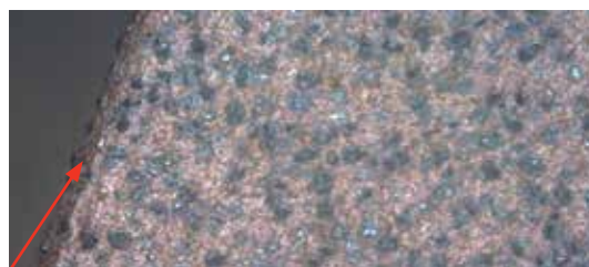
Exposed diamond grit (free cutting)
