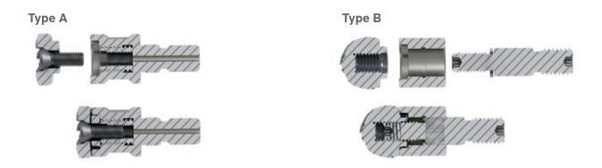
Threaded-end adapters are also used in threaded-end shanks which are commonly available on the market and also for extensions in cemented carbide. As there are different types of blanks, two types of adapters are required.
