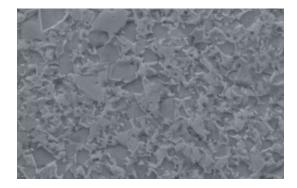
CTS20D for universal machining of alloyed and non-alloyed steels. Suitable for a variety of cutting operations on different materials thanks to its balanced properties. Improved toughness ensures a low risk of cutting edge breakage
