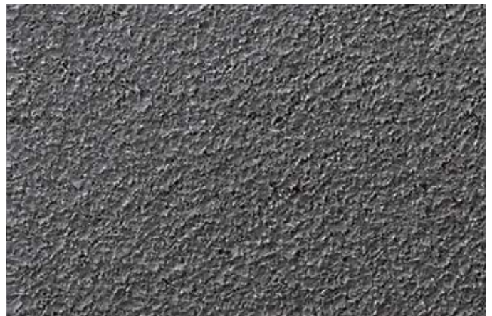
Micrograph of a WC Co cemented carbide surface after the ninth consecutive EDM cut in oil. 1) (Ra= 0.06 µm)
