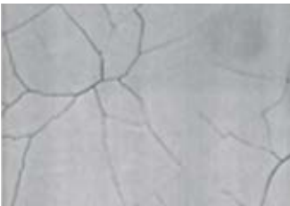
Possible effect of insufficient cooling
