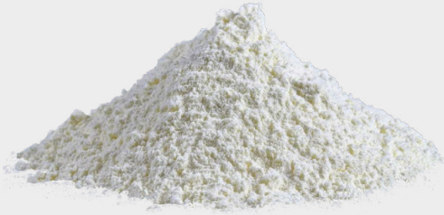
Boron nitride with a hexagonal lattice structure
